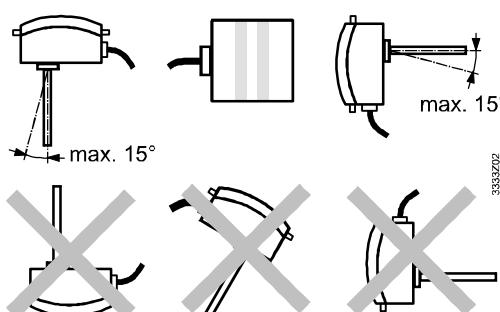
The controller may not be mounted upside down and the cable may not enter from the top.
