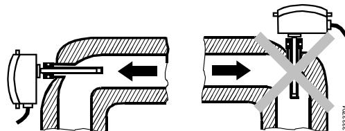
The controller should be mounted in a pipe bend with the protection pocket facing the flow.
